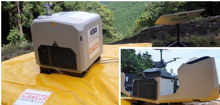
A drone with an automatic charging port and Starlink. The drone flies from the charging port by remote control and returns to the charging port after taking pictures..
