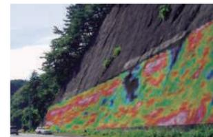
Analysis method: thermal infrared radiation imaging method, flexural oscillation method and coring method (combined use depending on the site conditions)
