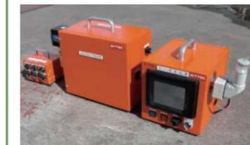
NITTOC's original system to control the flow volume of base and plastic materials based on the planned mixture.
