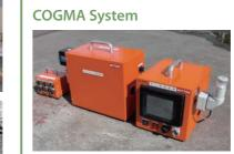
NITTOC's original system to control the flow volume of base and plastic materials based on the planned mixture
