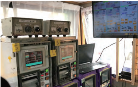
Flow rates and pressures can be checked on an office monitor.
