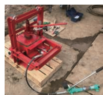
← On-site surface shear testing machine
