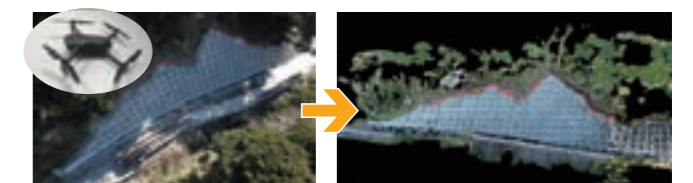
Slope surface photographed by drone → Creation of a 3D model from the photo
