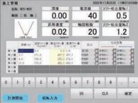
The machine operator's monitor displays information necessary for installation in real-time, which can be shared with remote site managers via the internet.
