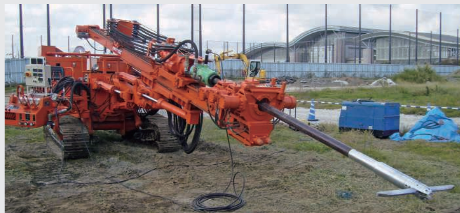
Mixing system with blades that can be expanded and retracted
