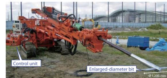
**Opposite Direction Mixing-Type Deep-Layer Mixing Method Compatible with Hard Ground**
