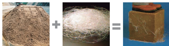
Sand from the left-side nozzle and polyester continuous fiber from the right-side nozzle are injected by jet water to form continuous fiber-reinforced soil.
