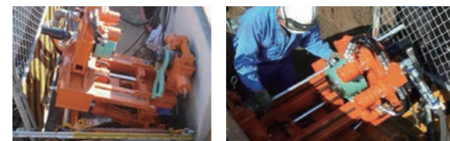
Drill machine is operable even with a clearance gap of only 1.5 m.
